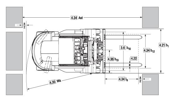
$$\begin{split} & \iota_{st} = \ Wa + x + I_6 + a \\ & \text{pplies only if} \quad \frac{b_{12}}{2} \le b_{13} \\ & \iota_{st} = \ Wa + \sqrt{(\ I_6 + x)^2 + \left(\frac{b_{12}}{2} - b_{13}\right)^2} + a \\ & \text{pplies only if} \quad \frac{b_{12}}{2} \ge b_{13} \\ & = 200 \end{split}$$
